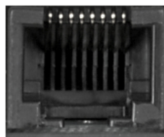
RJ45 connector for new Spiders without Tibbo: port 1001
